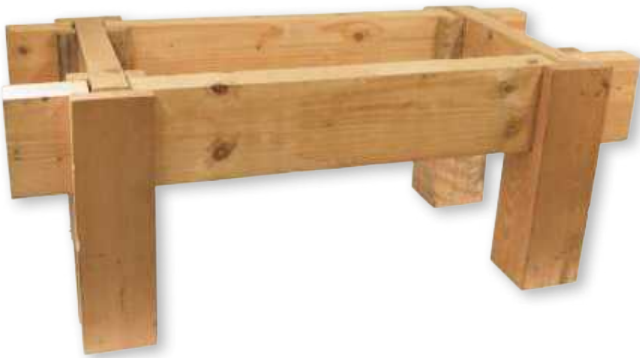
▲ Pic.10 A table base with interlocking joints. The big, flat surfaces would make this very strong if the long-grain mating surfaces were glued and pegged, although that was not the original design concept
